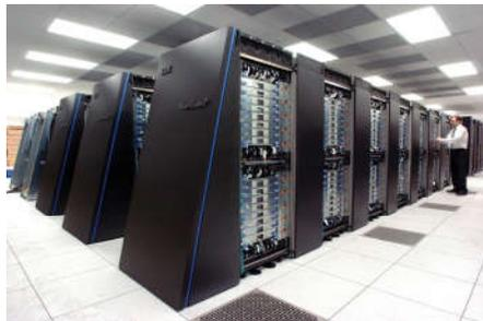
It was first delivered to the Lawrence Livermore National Laboratory in 2011 and now full deployed with an impressive 16.32 Petaflop/s on the Linpack benchmark using **1,572,864** cores.
